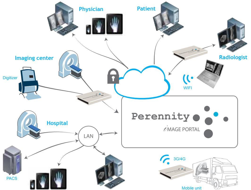
DICOM images, videos and reports are uploaded to the iIMAGE Portal server directly from modalities, workstations or PACS. The server can be either installed in the hospital facilities or hosted by an Internet Service Provider. All transfers are securely encrypted and the data is lossless compressed for fast transmission.
