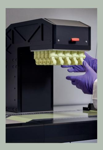
Featuring a large build volume and the unique capability of 3D printing both advanced ceramics and metals on one machine, optimized for high precision casting applications of silica shells and cores.
